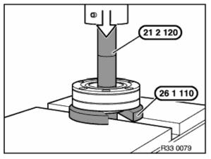
Special tool 26 1 110 must be used in accordance with diameter of output shaft. Bearing inner race must rest on rib of special tool.
